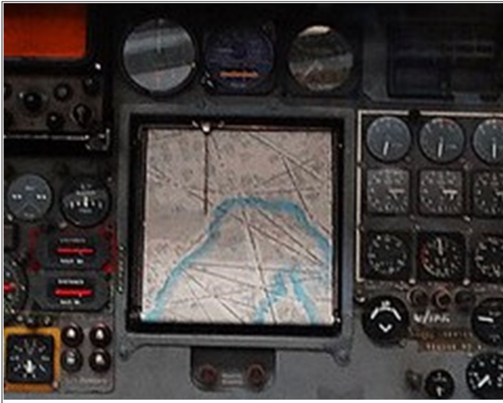
The map display with a paper route map fitted. Also clearly seen is the pointer, originally these had a pen nib on the end which drew a line on the map to show the route the aeroplane had flown. This was not very successful and also the maps could not be reused so the nib was removed. Photo: Steve Hall
