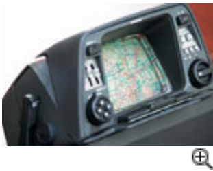
Honda's Electro Gyrocomator-the world's first navigation system for use in a car
