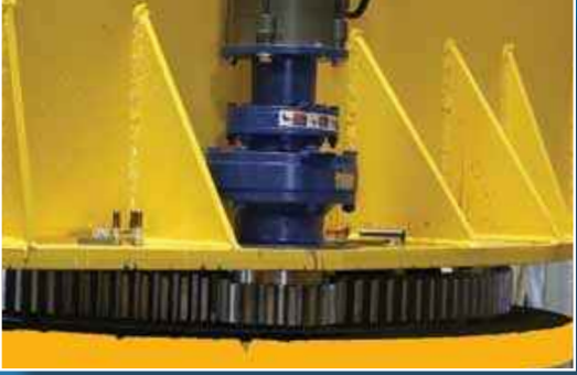
Slewing bearing, pinion gear and cyclo-drive gearmotor
