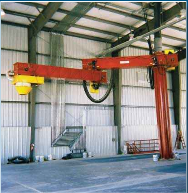
Post-mounted drag conveyor loader for DDGS
