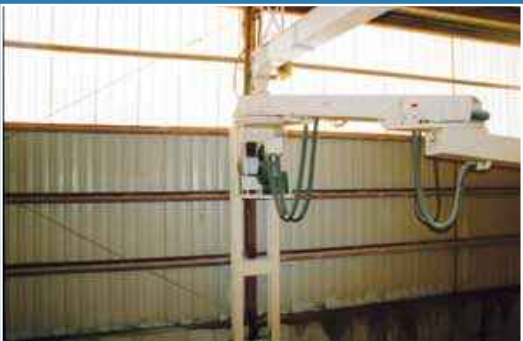
Post, platform or haunch mount (haunch mount shown)
