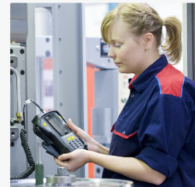
Condition monitoring systems
