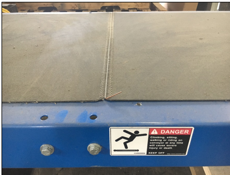
Figure 4 – Belt Ends Laced Together on Top of Conveyor
