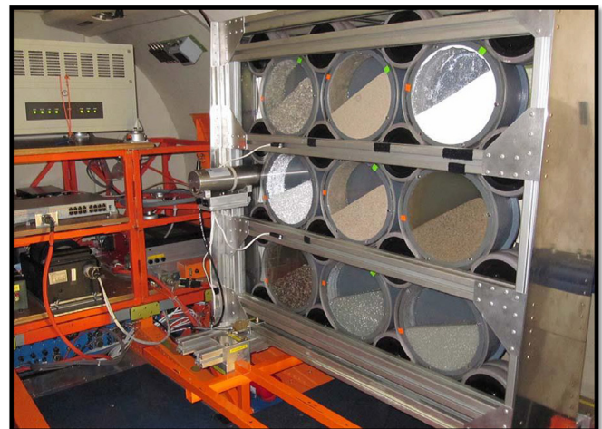
Fig. 18. Revolving cylinders housed in an airplane to measure the angle of repose under low gravity [46].
