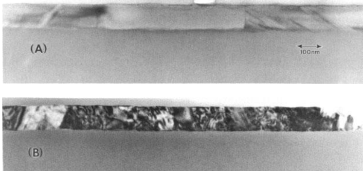
Fig. 3.2a,b. TEM cross section of two low-temperature processed poly-Si films on glass, providing a comparison of typical grains from (a) an excimer laser-crystallized film and (b) a thermally-crystallized film [3.31]
