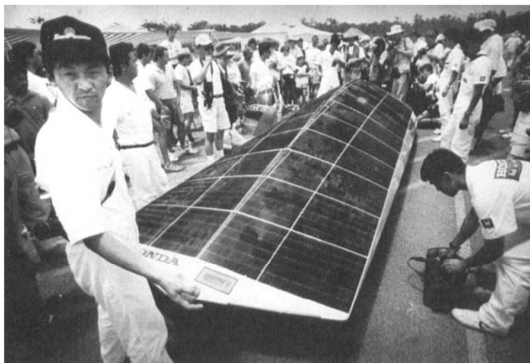
Figure 7. A rear view of the Honda Dream , showing particularly its solar array (photograph: M. H. Brown)
