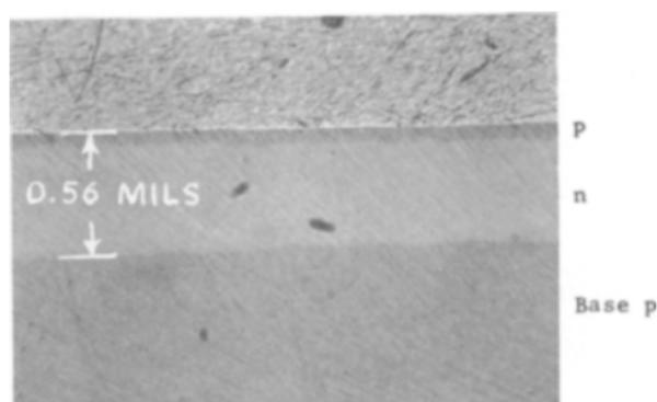
Fig. 2. Typical effect of various surface treatments on the formation of the \text{SiO}_4^+ complex from oxygen diffused into 54 ohm-cm p-type Si at 1250^\circ\text{C} for 3 hr, 250^\circ\text{C}/\text{hr} cooling rate; after 72 hr anneal at 450^\circ\text{C} ; beveled X-section depth magnified 10X. Microscope 60X.(a) Chemically polished surface.
