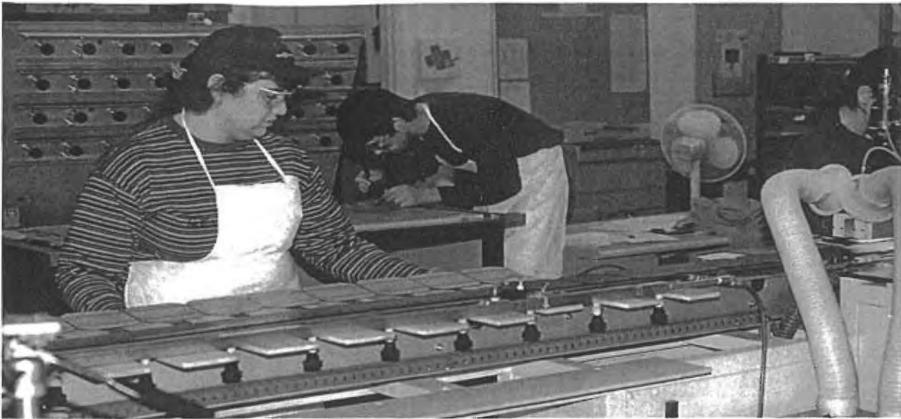
Figure 2.7. Assembling solar cells into strings. (AstroPower, Newark, DE)
