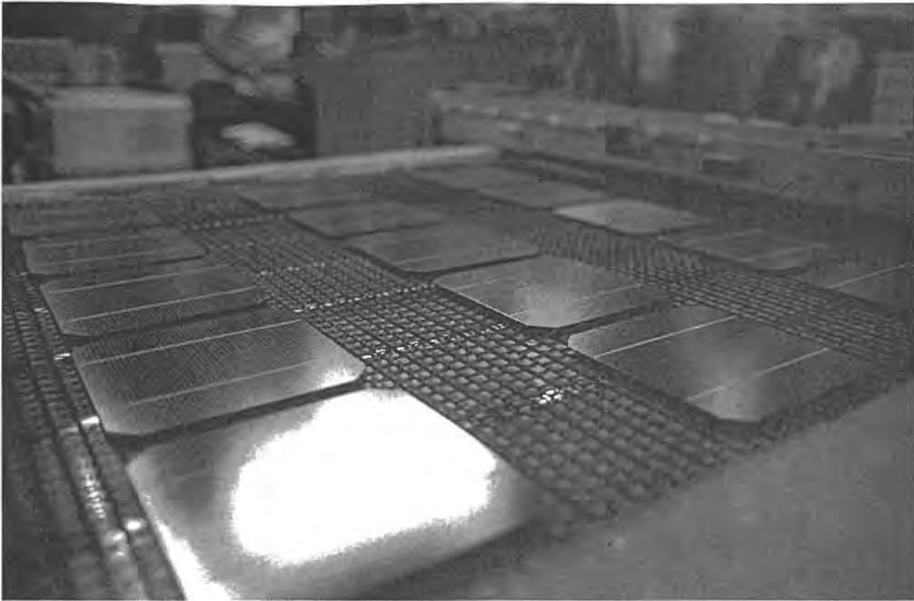
Figure 3.2. Finished AstroPower solar cells exiting the furnace where the top finger contacts were fused onto the single crystal silicon.
