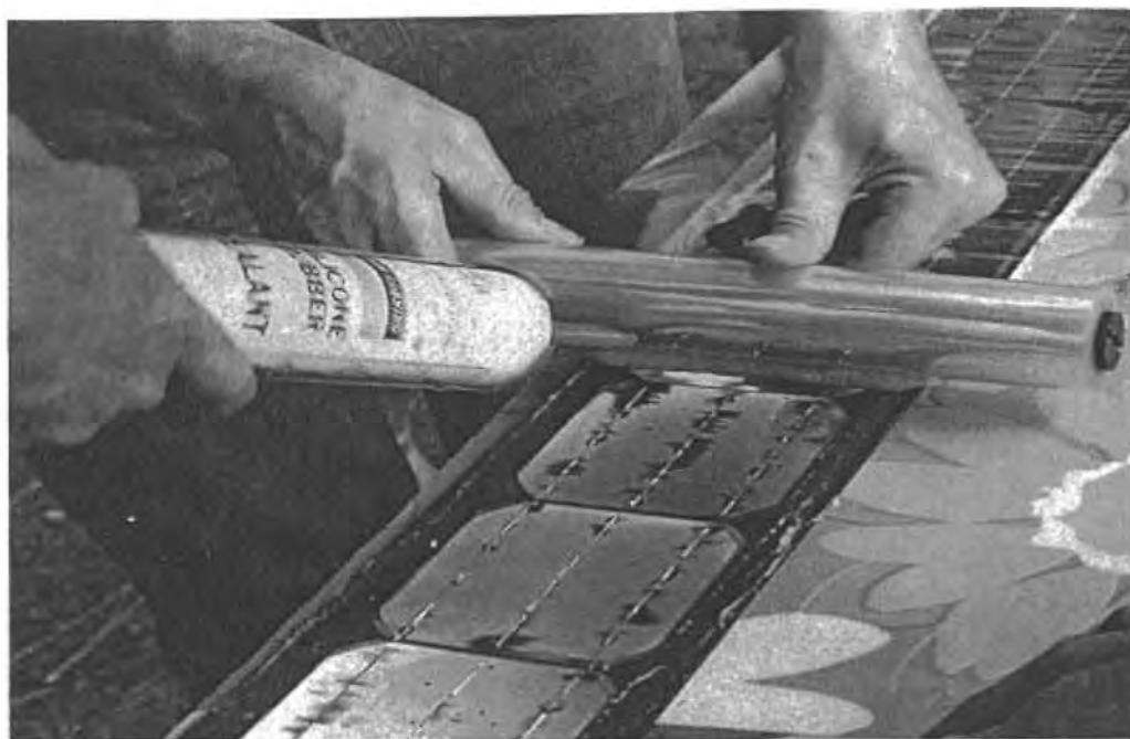
Figure A.12. Coating the top of the cells with silicone and Mylar film. The film presses out a bead of silicone RTV, eliminating voids and air bubbles. (Remote Power, Fort Collins, CO)
