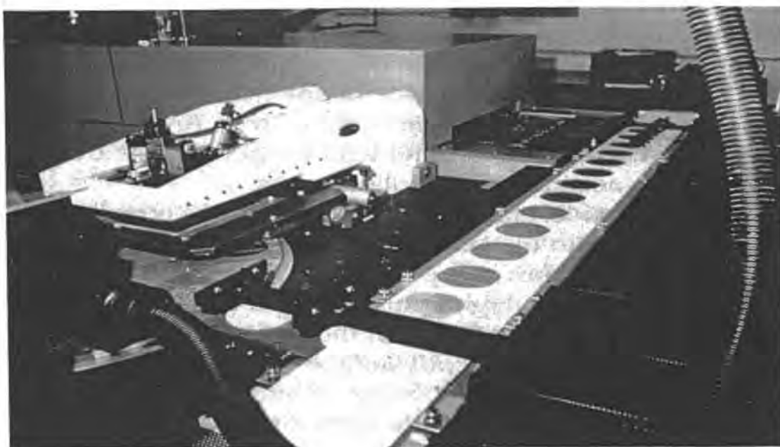
Figure 2.6. Automatic machinery soldering leads onto individual solar cells. These machines can replace tedious hand-soldering and produce a better joint. (Siemens Solar Industries, Camarillo, CA)
