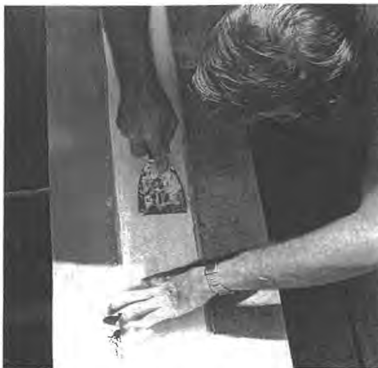
Figure A.10. Smoothing out a new layer of silicone over the cloth, completely embedding the cloth. (Skyheat Workshop photo)
