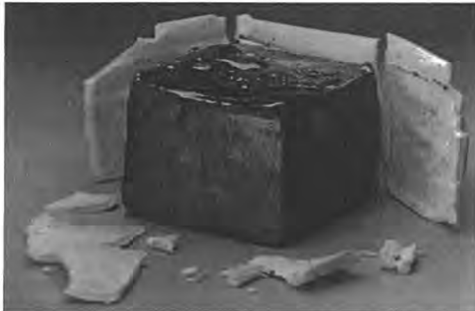
Figure 2.10. Heat exchanger method (HEM) single-crystal silicon ingot. (Crystal Systems, Salem, MA)
