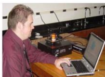
Ken Causey, a second-year student in the nanotechnology program at Forsyth Tech, navigates over graphite and gold surfaces with a NanoSurf EasyScan2 Atomic-Force Microscope.
