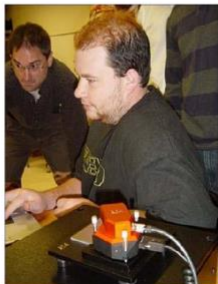
Faculty member Kevin Conley looks on as Corey Whitt, a second-year nanotech student, measures nanoscale features of a silicon surface with an atomic-force microscope.
