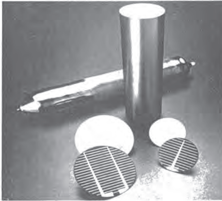
Figure 1.1. Silicon ingot, cylinder, wafers, and finished solar cells. (Jet Propulsion Laboratory, California Institute of Technology)
