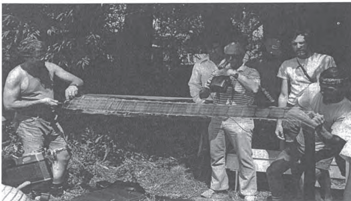
Figure A.13. The finished product is a completely encapsulated set of solar cells. (Remote Power, Fort Collins, CO)
