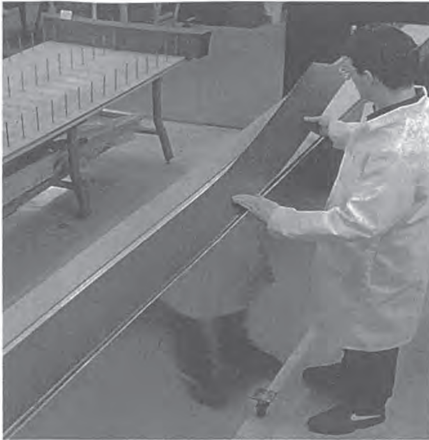
Figure 2.12. A thin film of crystalline silicon is grown on a proprietary substrate to make low-cost solar cells. (AstroPower, Newark, DE)
