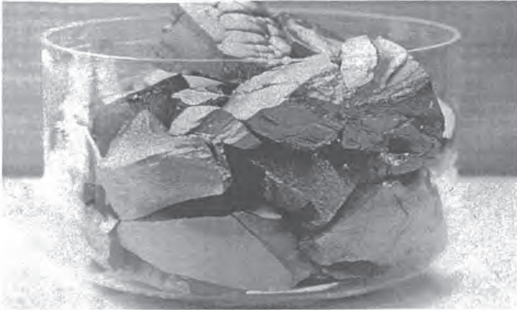
Figure 2.1. Semiconductor-grade silicon. This highly refined material is purer than fine gold and is becoming more expensive as supplies fail to keep up with demand. (Siemens Solar Industries, Camarillo, CA)
