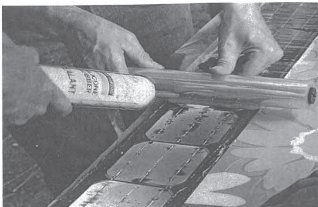
Figure A.12. Coating the top of the cells with silicone and Mylar film. The film presses out a bead of silicone RTV, eliminating voids and air bubbles. (Remote Power, Fort Collins, CO)
