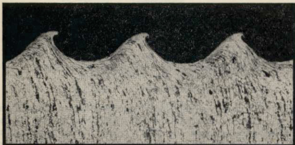
FIG. 2. Photomicrograph of a cross section of a projectile which shows the wave structure formed by 45 deg impact on a 0.010-in. lead target. The average distance from crest to crest is 0.033 in.
