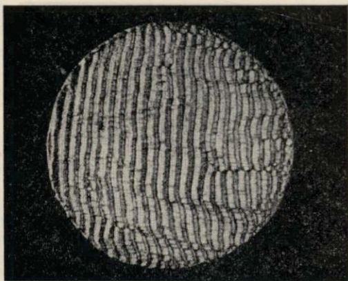
FIG. 1. End view of 0.50 caliber cylindrical steel projectile after it has passed through a 0.005-in. lead target at 45 deg striking angle. The actual diameter of this cylinder is 0.428 in.
