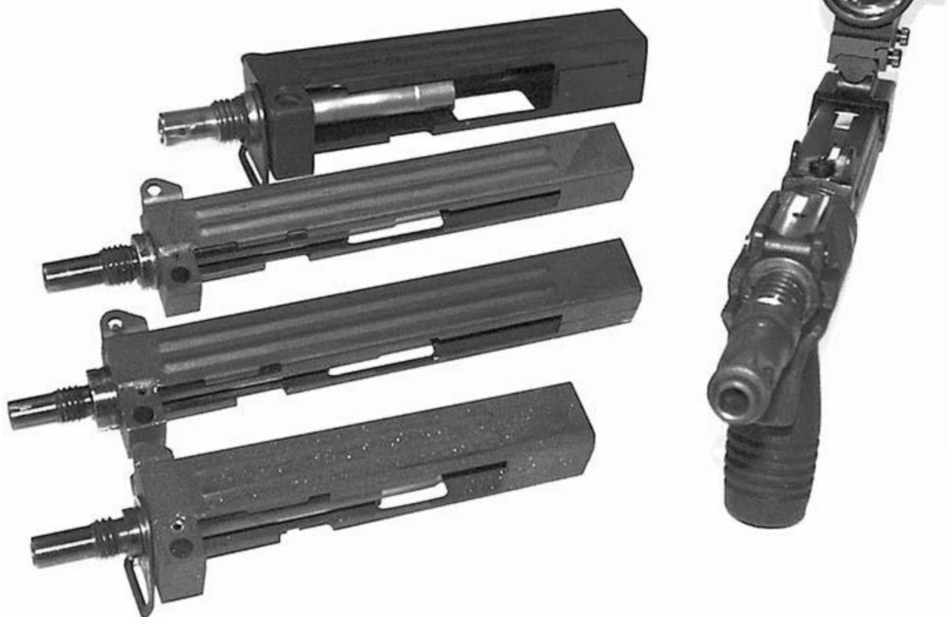
MAC upper assemblies. From top to bottom: MAC-10/45, SWD M11/380 "SlowFire" upper, SWD M11/9 upper, SWD M11A1 upper, and to the right a TASK/SlowFire M11/9 upper.
