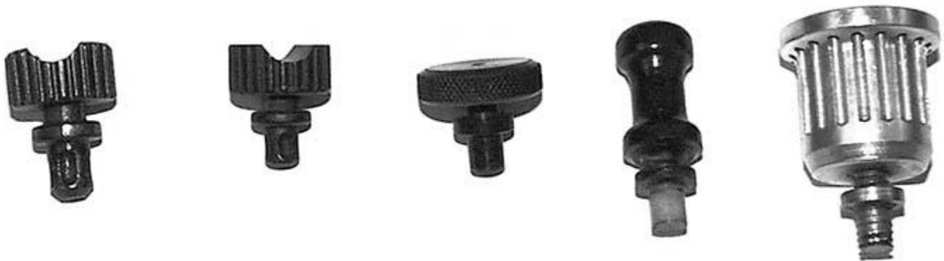
Different cocking knobs used for the MAC-type weapons. From left to right: MAC-10 cocking knob, SWD M11A1 cocking knob, SWD M11/9 cocking knob, author designed cocking knob made from Delrin, author designed cocking knob made from aluminum.
