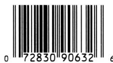
Figure 1: An example UPC barcode in the UPC-A format.
