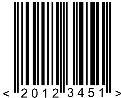
Figure 2: EAN-8 bar code symbol
