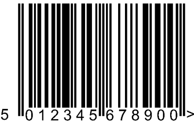
Figure 1: EAN-13 bar code symbol
