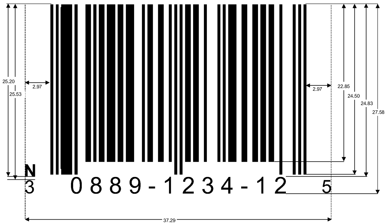
Figure E.3: UPC-A Example Variation
