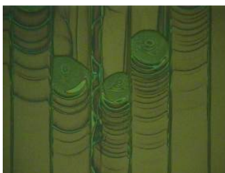
Figure 5.40: PEDOT printing defects in samples with 500 micron wide lines.
