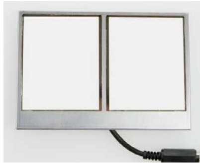
Figure 6.4: Final first year deliverable consisted of two white emitting tiles driven by the single pixel driver board and framed by a stainless steel bezel.
