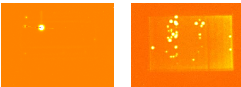
Figure 5.34: IR images of a spin coated (left) and printed sample (right). Bright spots are seen at points of high leakage.
