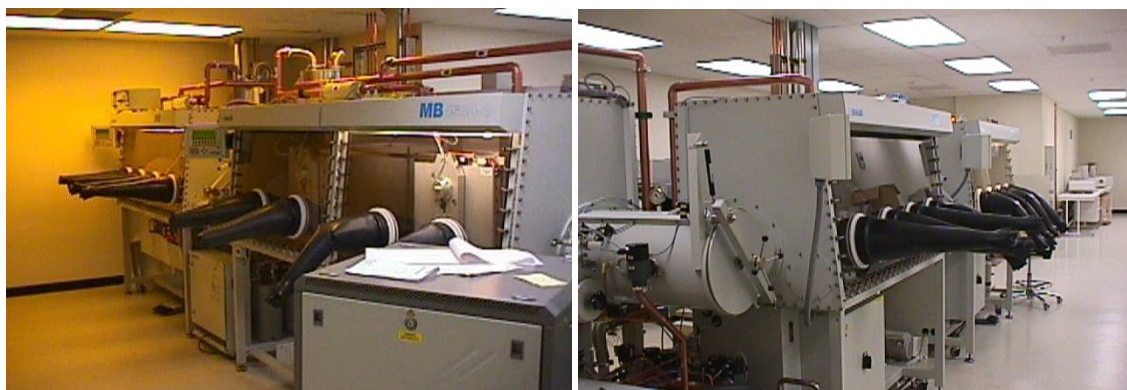
Figure 2.1: Inter-connected glove boxes; used for fabricating multiple small area OLED device for materials characterization and device testing.
