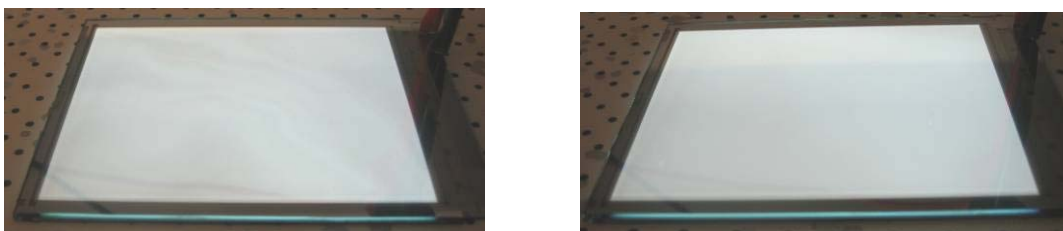
Figure 4.2: Wavy pattern in luminance due to non-uniformity in the light emitting polymer layer (left). Improved uniformity achieved by optimizing drying conditions (right).
