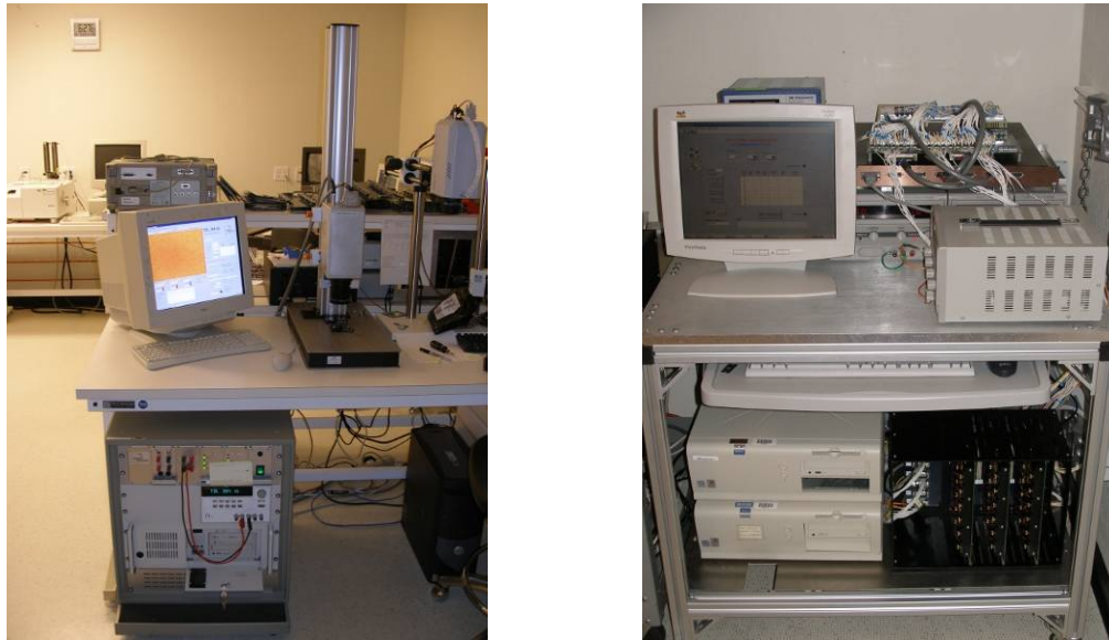
Figure 2.5: Infra-red imaging system (left) and Luminance Lifetime measurement system (right) used for reliability testing.
