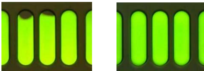
Figure 5.20: Photoluminescence images showing pockets with mouse-bites (left), and pockets without mouse-bites (right) printed with the new optimized process.
