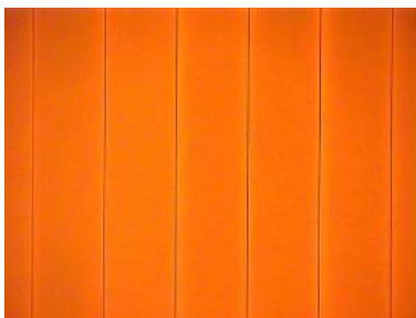
Figure 5.41: A sample with very high fill factor (>90%) with optimal PEDOT and LEP printing.
