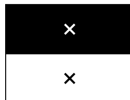
Figure 3.14 The test screen for lifetime measurement. The marks indicate the position of the spectroradiometer.
