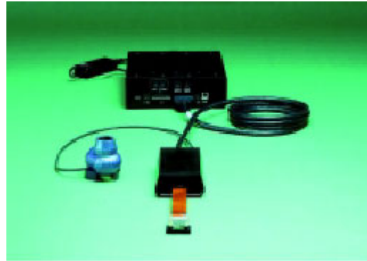
Figure 3.3 The CRL Opto LCOS evaluation kit.
