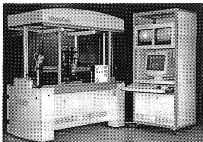
Figure 4. Jetlab® printing station for direct writing from data files of patterns of micro-optical, adhesive, solder or biomedical elements, and consisting of print head(s), XYZ stages, drive electronics, software and pneumatic & temperature controls.
