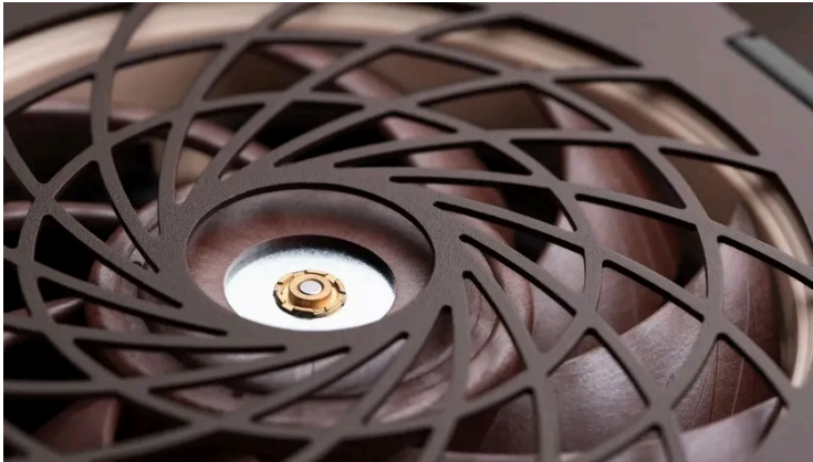
Noctua shares a fan grill design that drops noise levels
