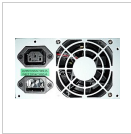
Some desktop computers provide both a C14 inlet (lower) and a type F outlet (upper) for powering the monitor
