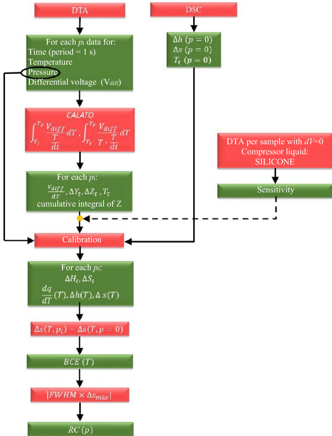
Figure 5.15. Diagram of the experimentation process to obtain the caloric effect.
