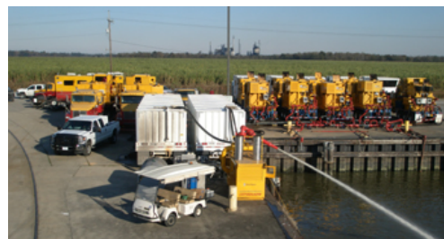
19,000 Frac HHP with two Blenders and a Data Van
