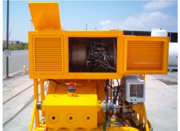
The 3,850 HP gas turbine stacked above the pumps weighs only 770 lbs.
