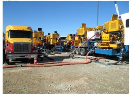
Frac job in East Texas. 19,000 HHP with 125 BPM Blender and Data Van.
