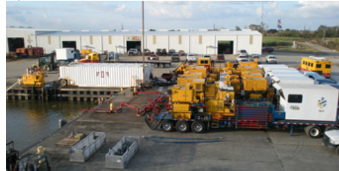
19,000 Frac HHP with two Blenders and a Data Van
