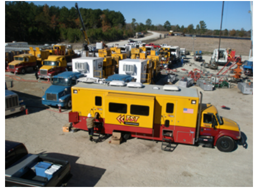
Frac job in East Texas. 19,000 HHP with 125 BPM Blender and Data Van.
