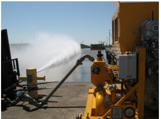
The 3,850 HP gas turbine stacked above the pumps weighs only 770 lbs.
