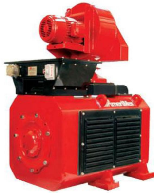
Figure 7—Electric motors replace diesel engines on the electric powered hydraulic fracturing fleet
