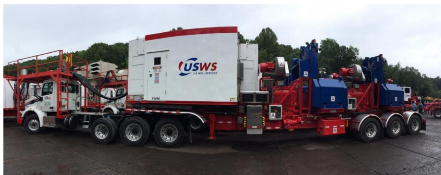
Figure 8—Dual hydraulic fracturing pump trailer, 3500 HHP
