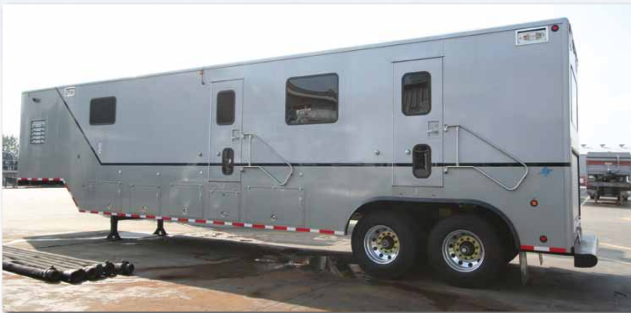
ET-40ACD Data van command center provides control of critical well site equipment.
