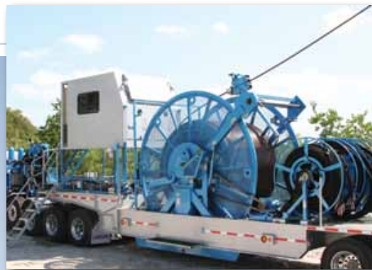
TT-100-XC Trailer-mounted high capacity coiled tubing unit.
