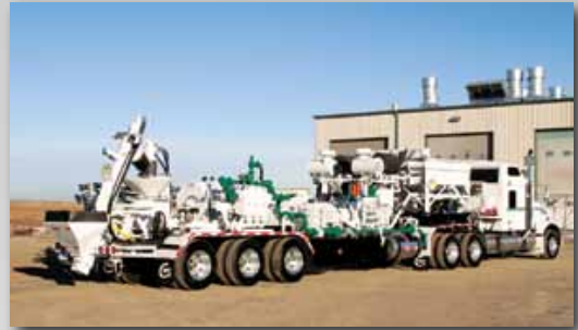
Combination fracturing pump and blender.
