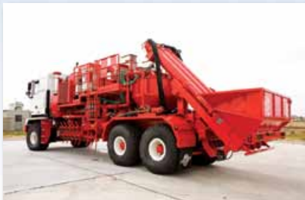
MC-60 Bodyload fracturing blender for extreme cold weather operations.
