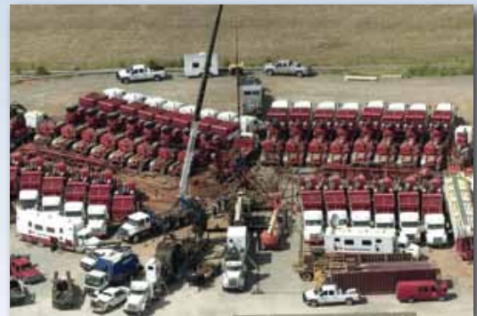
Stewart & Stevenson's integrated fracturing equipment on a dual simultaneous fracturing job.
