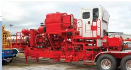
WT-601 Single pump trailer with control cabin.
