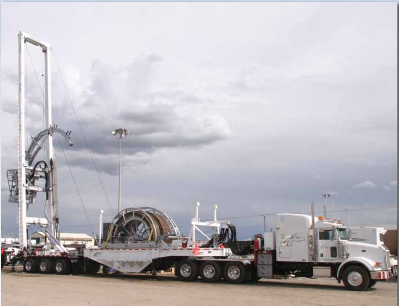
Masted coiled tubing unit.
