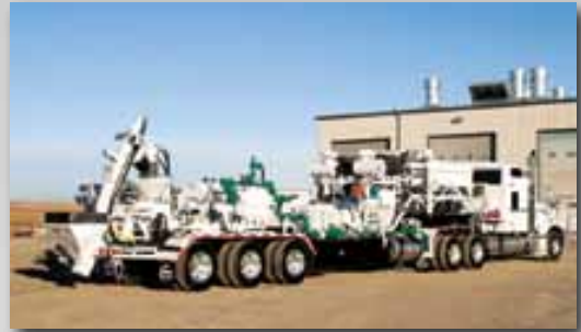
Combination fracturing pump and blender.
