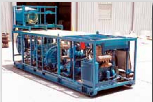
Skid mounted acid injection system.
