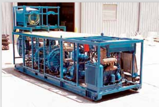
Skid mounted acid injection system.
