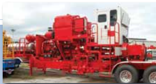
WT-601 Single pump trailer with control cabin.
