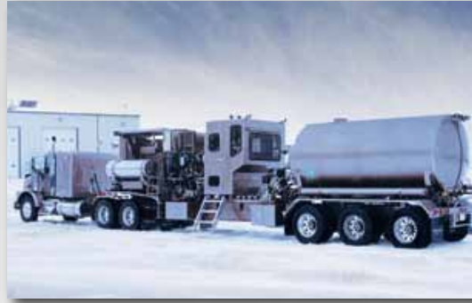
NT-181-NF 180K SCFH Trailer nitrogen unit with control cabin.
