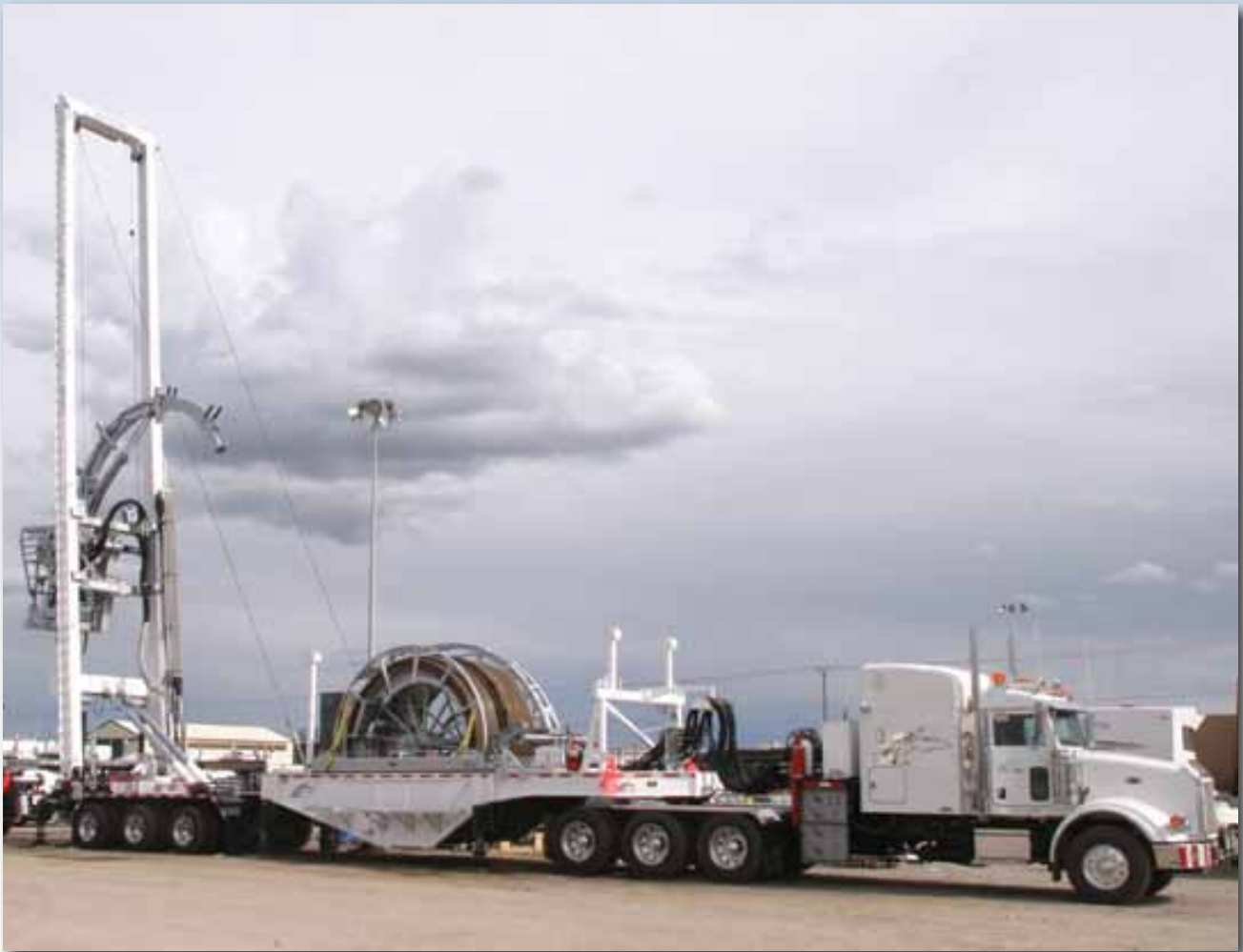
Masted coiled tubing unit.
