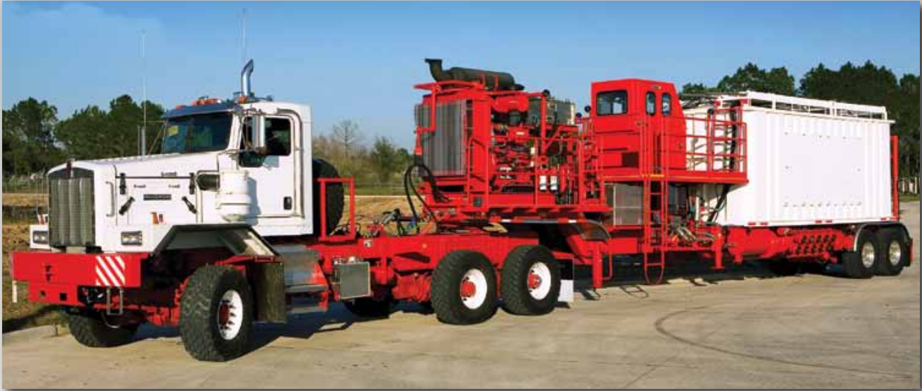
CT-5CAS/BT-200 Trailer mounted chemical additive and hydration unit.
