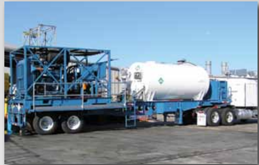
NS-181-NF 180K SCFH Nitrogen skid on a trailer.
