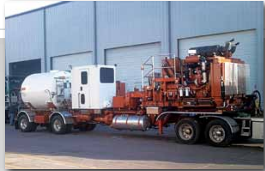
WNT-601-181-NF Combination nitrogen and fluid pumper.
