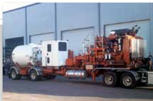
WNT-601-181-NF Combination nitrogen and fluid pumper.
