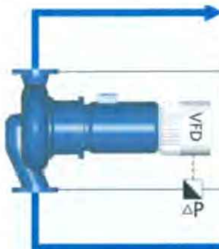
Figure 8.10: Circulation pump with differential pressure sensor
