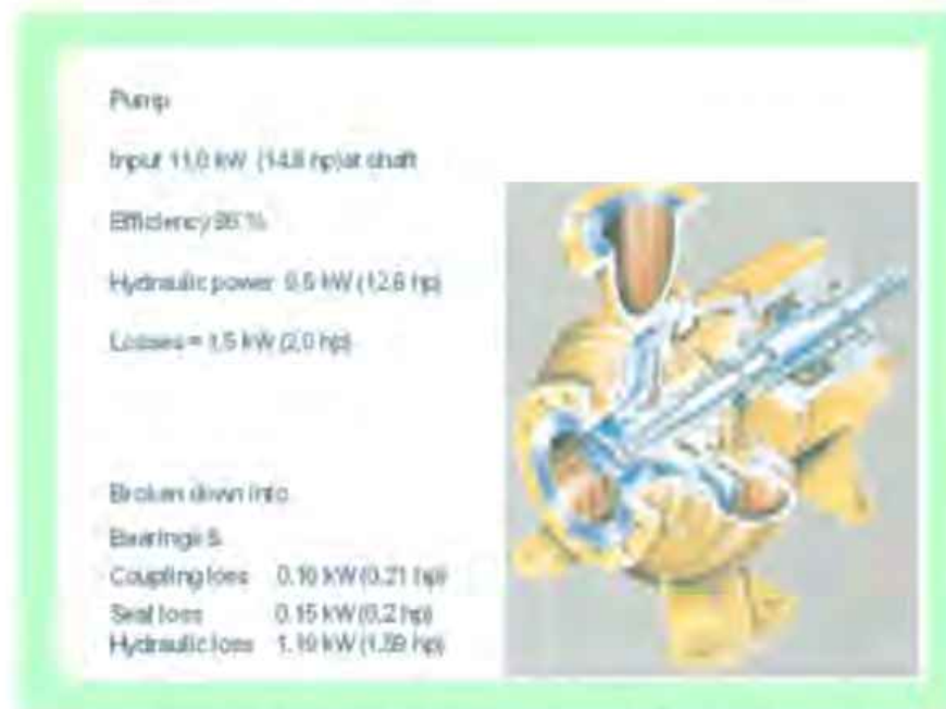
Figure A6.2: Typical rotodynamic pump losses
