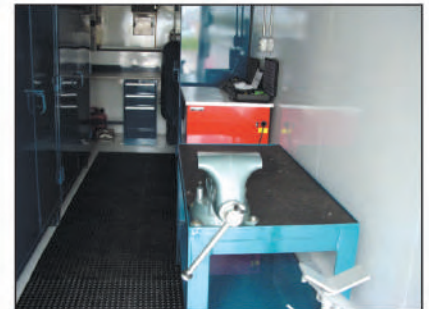
Work table and vise for disassembly, re kitting, and re assembly; Ample storage space for parts kits; ¼ ton hoist and jib crane; Wash vat for cleaning parts
