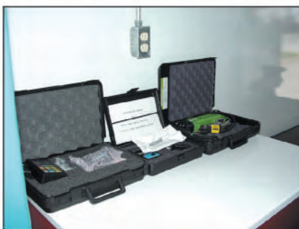
Magnetic Particle Inspection, yoke style with spray fluid and black light.
