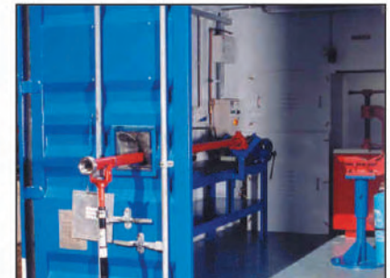
Port hole allows pipe to extend beyond the length of the trailer during poor weather conditions.
