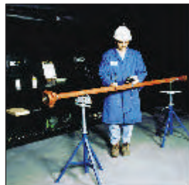
Step 2: Wall Thickness
