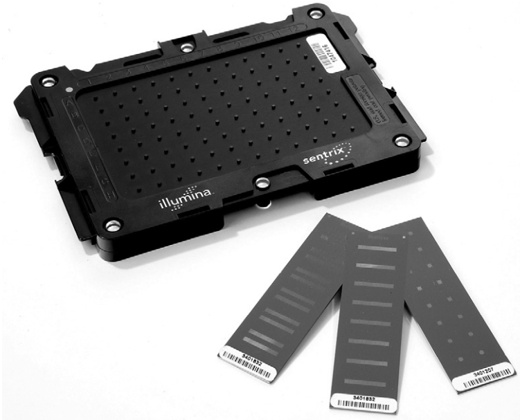
FIG. 2. Two different Array of Arrays formats: the 96-sample Sentrix Array Matrix (SAM) and the multisample Sentrix BeadChip. The SAM substrate (upper) is composed of 96 arrays. Each array is composed of ~50,000 fiber-optic strands chemically etched to create a well for a single bead. The BeadChip formats (lower) feature flexible configuration with dense packing ratios that can be used for 1 to 16 samples per BeadChip.
