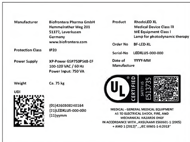
Figure 21: Product label (serial number and date of manufacturing vary) with UDI code of RhodoLED ® XL on lamp base, individual code depends on the serial number and date of manufacturing of the device.
