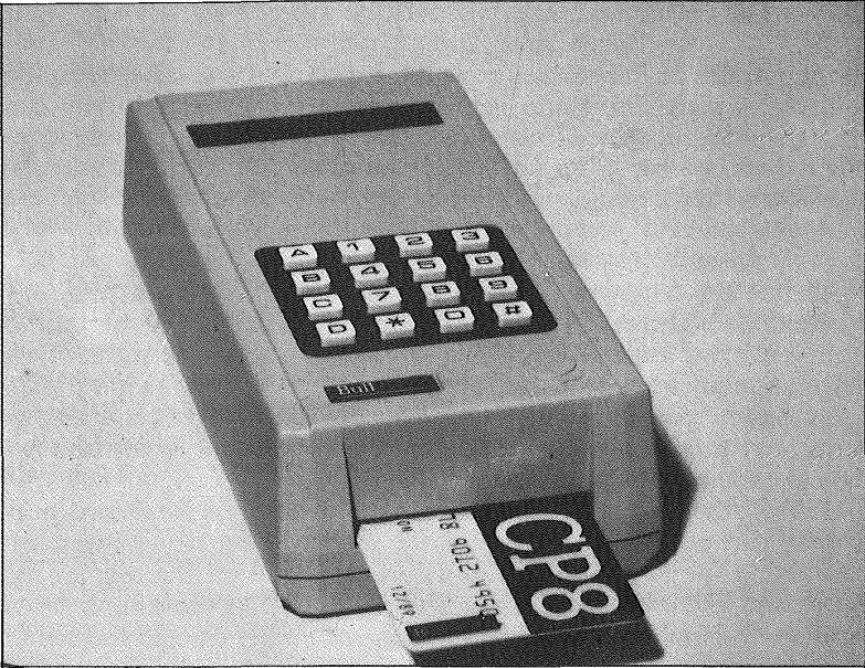
Fig. 3.4. Portable contact smart card read/write unit. It is battery powered although it can also be powered from the mains. (Photograph courtesy of Bull CP8)
