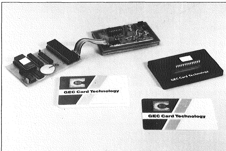
Fig. 2.2. Stages of card development that have led to an ISO standard GEC contactless smart card. From top to bottom: the printed circuit prototype comprising two boards; a 5mm thick card with a protruding EPROM which could be removed for reprogramming; a 5mm thick card which could be reprogrammed from the read/write unit; the ISO standard card. (Photograph courtesy of GEC)
