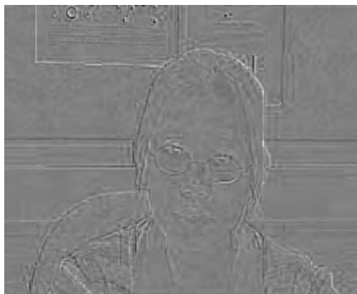
Figure 5.61 Residual to be encoded as enhancement layer
