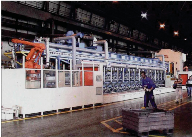
Figure 1: Press hardening line for B-pillars of a mass- produced automobile
