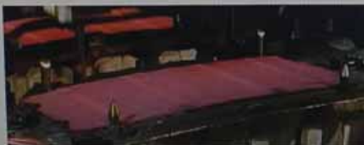
Figure 20a: Blank just before stamping
