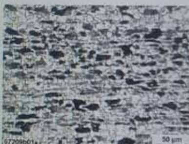
Figure 3: Typical HSM ferrite-pearlite microstructure.
