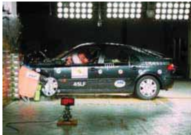
figure 24 : EuroNcap front crash of the LAGUNA II
