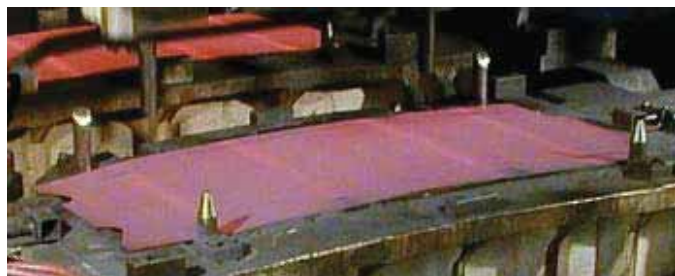
figure 20a: Blank just before stamping
