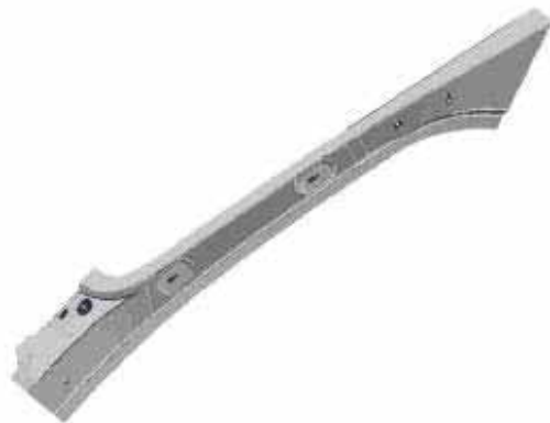
Figure 21 : C5 A frame reinforcement
