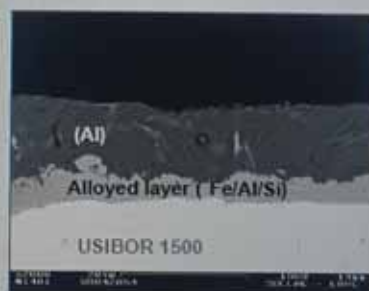
Figure 4: Typical microstructure of coating section by BSE on an SEM.
