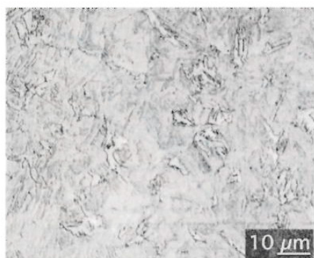
Fig. 10. Ferrite (about 6%) among martensite after the plastic strain of 0.04 at 800°C and cooling at 50°C/s.
