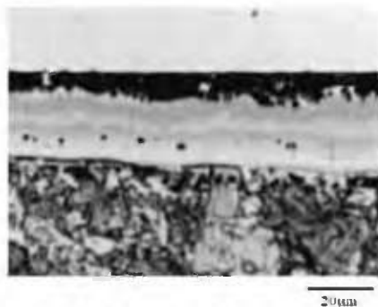
Fig. 12 Sectional optical micrograph showing plating layer structure after heated at 950°C for 30 s
