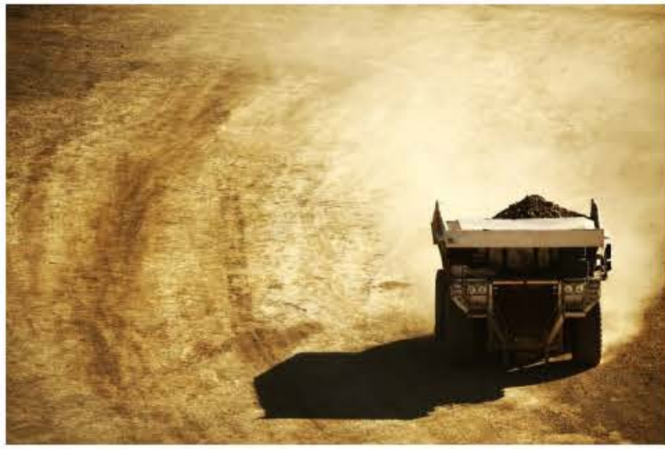
Haul Trucks Deliver ROM Ore to Crusher Hoppers
