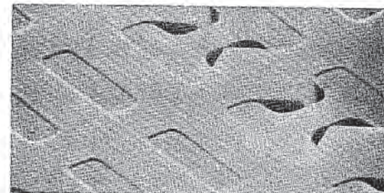
Fig. 2-42 Corner faceting problem that occurs during selective epitaxial growth in oxide windows. 70 Reprinted with permission of Solid State Technology.
