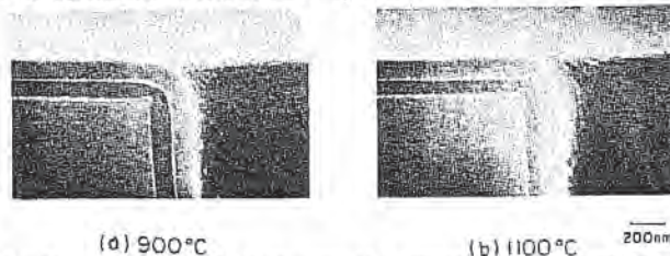
Fig. 2-38, Cross-sectional SEM photograph of a convex corner after oxidation in dry \text{O}_2 ambient. 60 (© 1987 IEEE).
