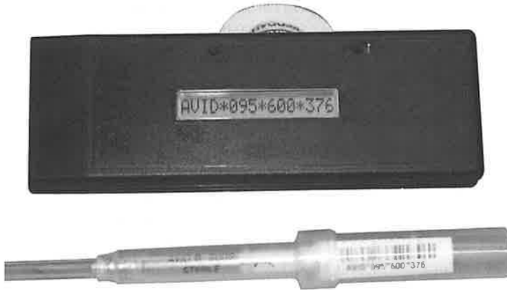
FIGURE 1-2 . A tag and reader (image courtesy of Merten G. Pearson, D.V.M.)
