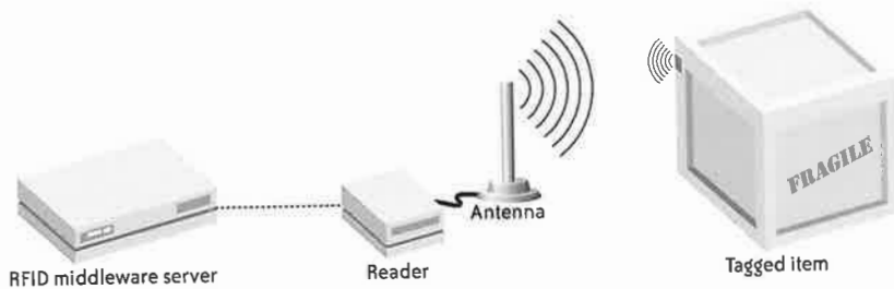
FIGURE 1-1. An RFID system
