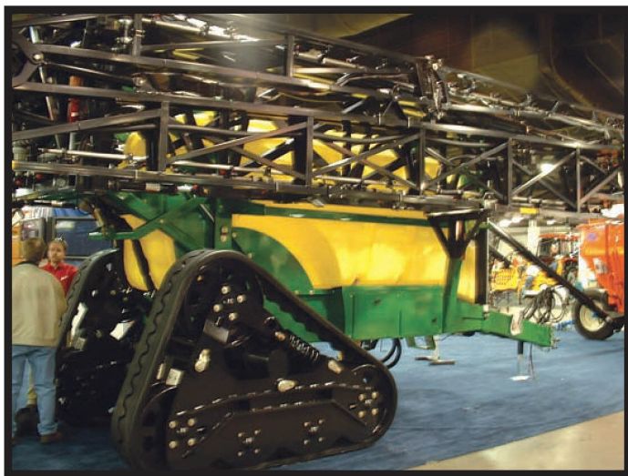
Chris Ayers (TM - KY, TN, S. IL) promoting the new, tracked undercarriage for Top Air 1600 and 2400 sprayers.
