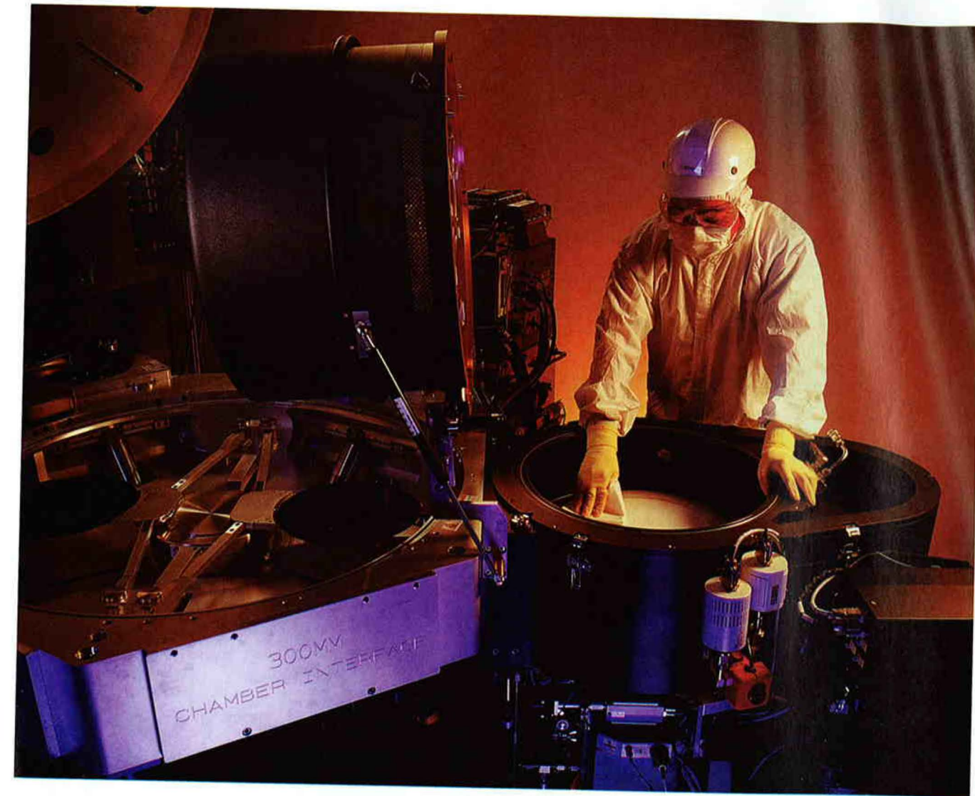
Servicing a 300-mm etch tool. Photograph courtesy of Applied Materials, Inc.
