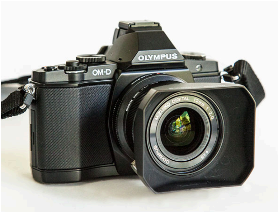
Rectangular lens hoods are often produced for wide-angle prime lenses like the M-Zuiko 12mm f/2.0, shown here on the Olympus OM-D E-M5 camera.
