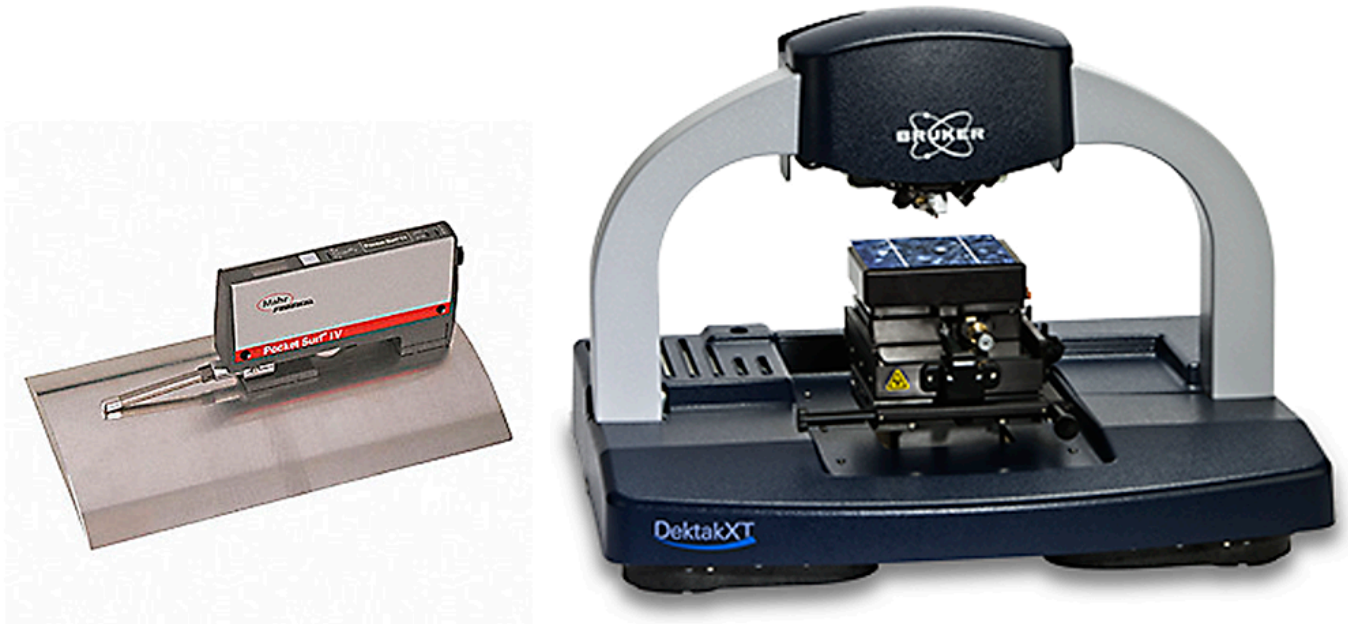
Stylus instruments range from hand held gauges to highly automated instruments.
