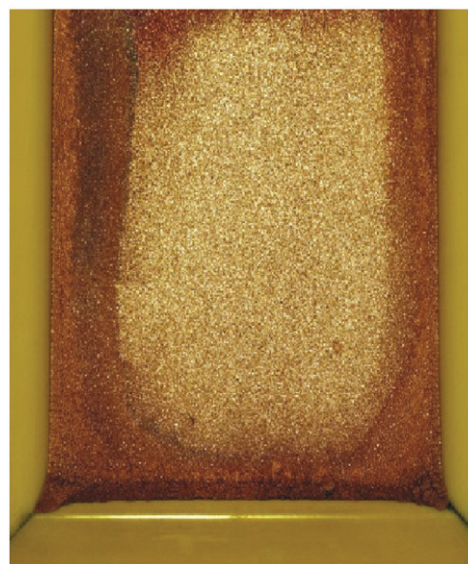
Fig. 9. Copper deposit obtained with APAM at 340 A/m 2 and 44 h and 35 min.
