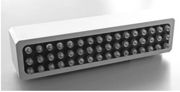
22.20 Ultrasonic array with 48 transducers in 16 groups.
