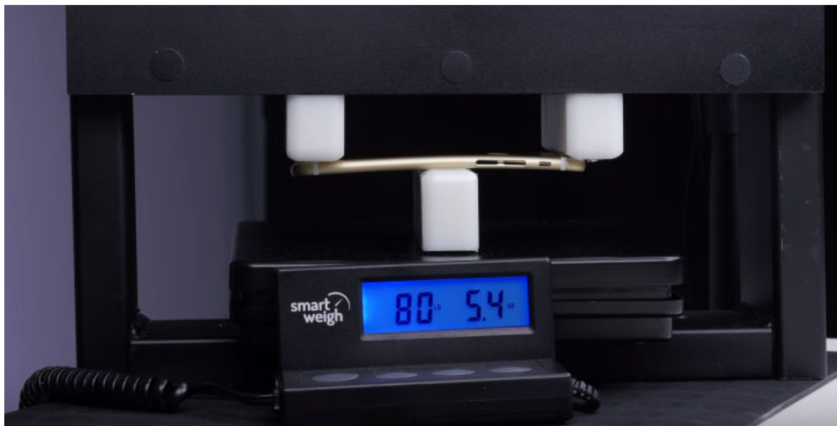
iPhone 6S chassis changes mean it can withstand up to 80lbs of pressure UNBOX THERAPY
