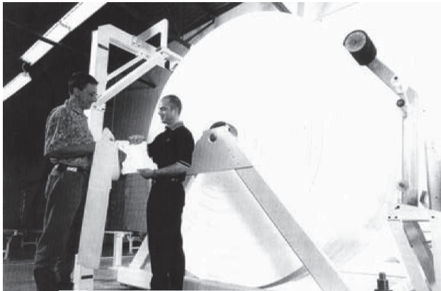
Fig. 8 'Superspool' concept for handling and shipping large rolls of absorbent products
