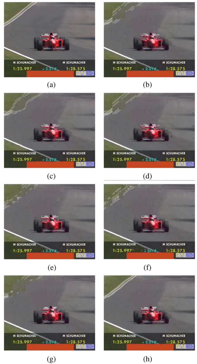
Fig. 12. Interpolated results of frame 56 of the Formula1 sequence using (a) original frame; (b) direct interpolation (PSNR: 29.68 dB, SSIM: 0.9050); (c) MV smoothing (PSNR: 29.46 dB, SSIM: 0.9013); (d) vector median filtering (PSNR: 29.80 dB, SSIM: 0.9067); (e) adaptive vector median filter (PSNR: 29.91 dB, SSIM: 0.9155); (f) multisize block matching algorithm (PSNR: 29.85 dB, SSIM: 0.9149); (g) proposed MV selection (PSNR: 30.23 dB, SSIM: 0.9225); and (h) the proposed multistage MV processing method (PSNR: 31.56 dB, SSIM: 0.9567), respectively.
