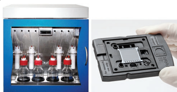
Figure 2 | The HybSelector instrument and a HybSelect Biochip for the selective enrichment of genomic target regions for next-generation sequencing.
