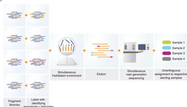
Figure 1 | High levels of multiplexing achieved by combining HybSelect™ parallel sample processing capabilities with bar-coding reagents. After automated sequence capture with HybSelect, targeted NGS was carried out on the SOLiD™ Sequencing System. The use of molecular barcodes allows the confident identification and tracking of samples
